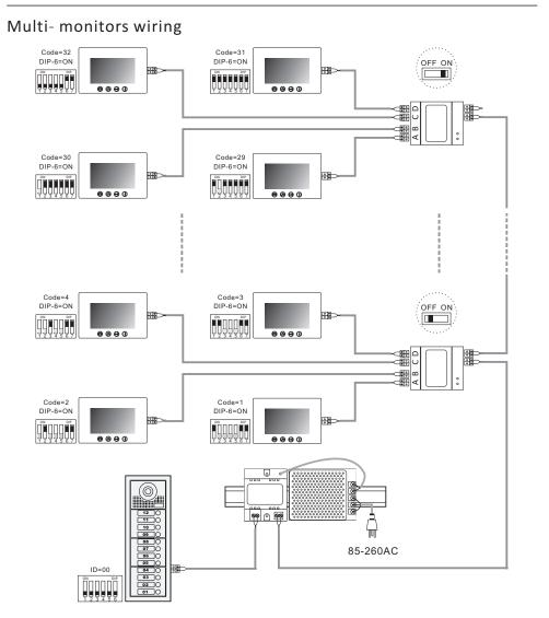
Power supply: Working Temperature: Wiring: Dimension: DC20~30V -10°C ~ +40°C 2-wires (Non-polarity) 89(H)×70(W)×45(D)mm
