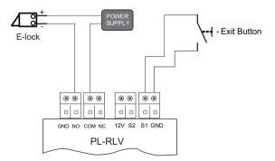
B: Power-off-to-unlock(fail-safe) lock:
