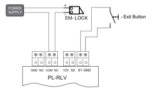
In a single system, two PL-RLV units can be connected to control a gate/lock and a light if required
