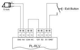
5.2 External Power Supply powered lock connection
