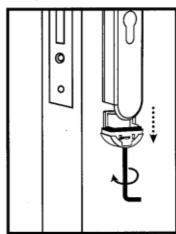
Use hexagon screw driver (#1.5) to pull out the battery holder from the bottom of the outer handle set.
