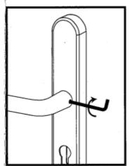
Take one hexagon driver (#2.5) to tighten the screw on the inner lever.
