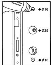
If there is an existing mortise lock, remove it before drilling.
