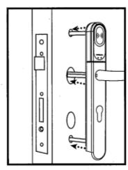
Insert the outer handle set into the holes on the door.
