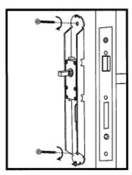
Take two screws and screw with the inner handle set on the door.
