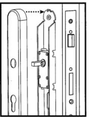
Put the inner handle cover plate back to the inner handle set.
