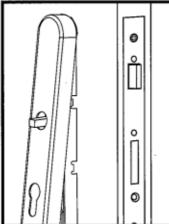
The cover plate should press to the surface of the door.
