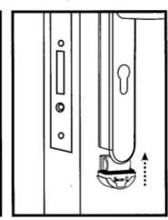
Insert one CR2 lithium battery to the battery holder and put the holder back.
