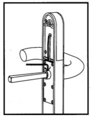
From the parts bag, take out the square spindle and place to the back of outer handle set.
