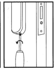
Garefully turn the screw at the bottom of the plate anticlockwise until you feel resistance.
